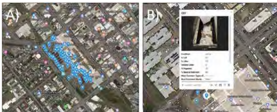
Figure 3. Using GIS (A) to map litter captured in at-source litter traps at a shopping centre allows for location-specific data such as discovering polystyrene foam packaging at loading docks (B)
